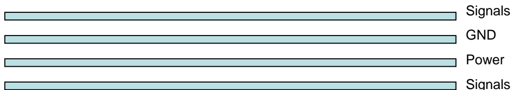
Figure 21: Typical 4-layer PCB construction
